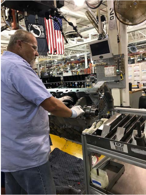
Machine operator installing crankshaft & bearings at the Detroit Diesel Factory
