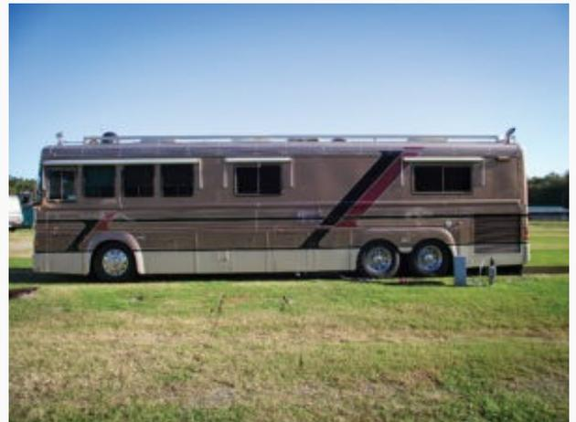
Stout construction materials include a 20-gauge steel roof, 14-gauge steel floor and 16-gauge steel side panels. The original exterior paint continues to shine.
