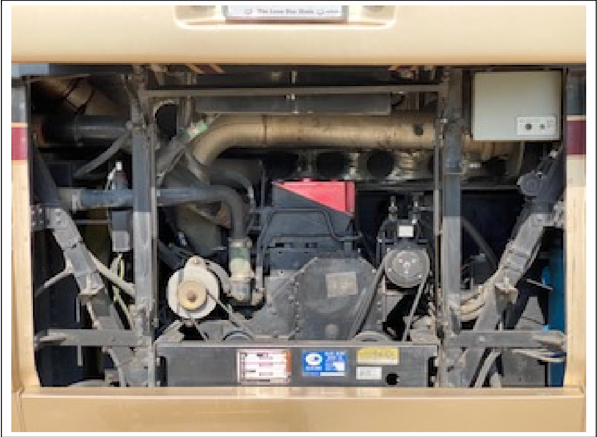
Photo # 5 Description: Cummins diesel engine
